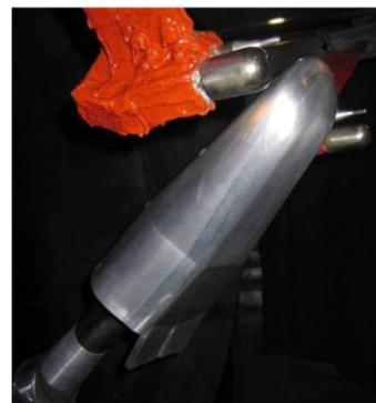
Fig 6: ONERA F4, IXV model in test section
