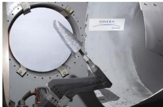
Fig 2: IXV model in the test section
